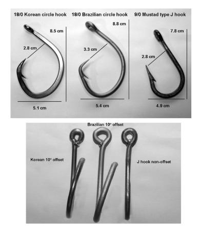
Figure 2. Lateral (above) and frontal (below) views of circle hooks 18/0,  $10^{\circ}$  offset (Korean-left, Brazilian – centre) and Mustad type 'J' hook 9/0,  $0^{\circ}$  offset – right. Photos: V. Fonseca.
