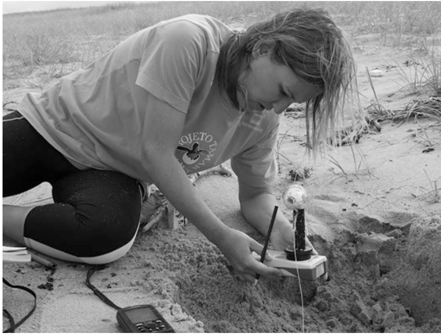
Fig. 7.16 Biologist collecting information on sand temperature in the field with a temperature datalogger
